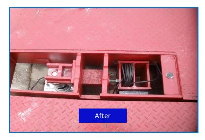
Weightron Bilanciai's patented technology converts Avery Weigh-Tronix Bridgemont weighbridges from existing Weigh Bar load cells to their stainless steel CPR and CPD canister load cells. The conversion process is extremely straightforward and can be carried out with the weighbridge in situ, thereby causing minimum site disruption.
