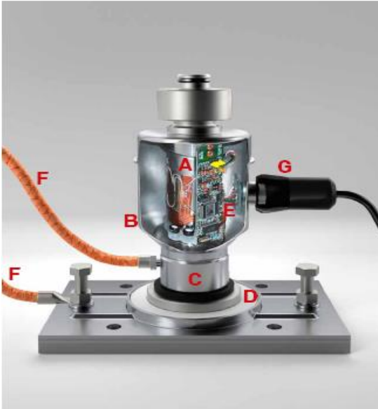
A - 8 STRAIN GAUGES High precision - Repeatability - Reproducibility B - HEAVY-DUTY PROTECTION AT 45° CONE C - MECHANICAL PROTECTION COVER D - INSULATION DISC FOR LIGHTNING PROTECTION E - OVERVOLTAGE AND INTERFERENCES PROTECTION F - COPPER BRAIDED EARTHING CABLE G - WATERTIGHT IP68/IP69K STAINLES STEEL CONNECTOR
