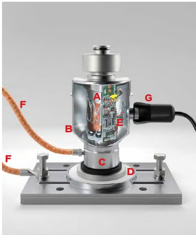
A - 8 STRAIN GAUGES High precision - Repeatability - Reproducibility B - HEAVY-DUTY PROTECTION AT 45° CONE C - MECHANICAL PROTECTION COVER D - INSULATION DISC FOR LIGHTNING PROTECTION E - OVERVOLTAGE AND INTERFERENCES PROTECTION F - COPPER BRAIDED EARTHING CABLE G - WATERTIGHT IP68/IP69K STAINLES STEEL CONNECTOR
